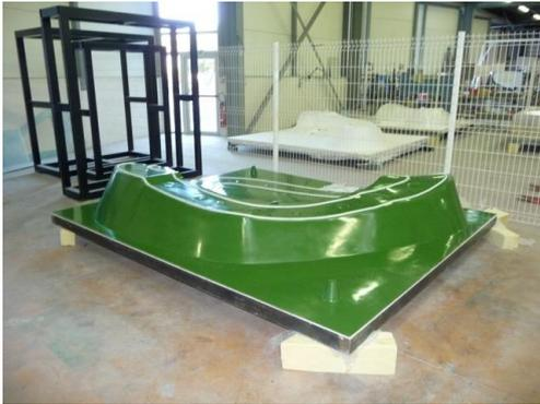
Considerable thought has gone into the design of the Air Pod to make it easy to build and maximise utilisation of every part by having multiple functions wherever possible. The moulded construction plays a big part in making this possible. It's good for achieving a low weight too!
